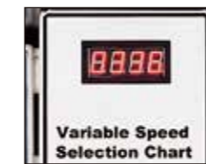
LED spindle rpm readout
