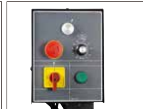
HB System Dual Function for RF-210V (Inverter Variable Manual & Hydraulic Cutting Speed Single Phase Only) (option for RF-210 only)
