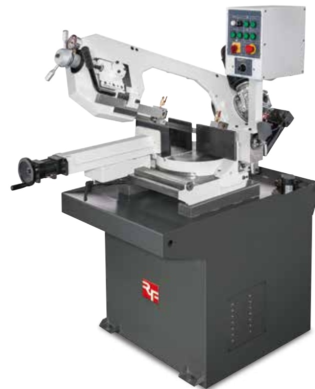
HB System Dual Function for Manual & Hydraulic Cutting (optional)
